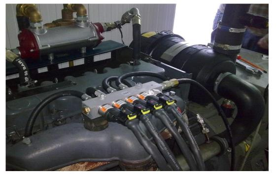
Dual fuelled hydrogen and biofuel CHP and Trigeneration
