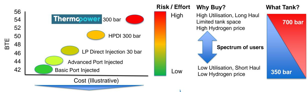
Efficiency driver is higher pressure, direct injection of Hydrogen into the engine.
