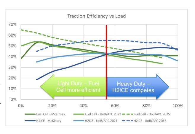
**Fuel Cell vs Hydrogen ICE:** Reports from McKinsey (2021) and APC / University of Brighton (2021) highlight how the higher loads of Heavy Duty might favour an efficient Hydrogen ICE
