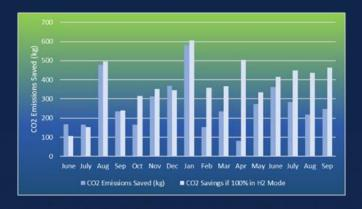
Dual-fuel retrofitting has the potential to save up to 40% of emissions compared to purely diesel vehicles
