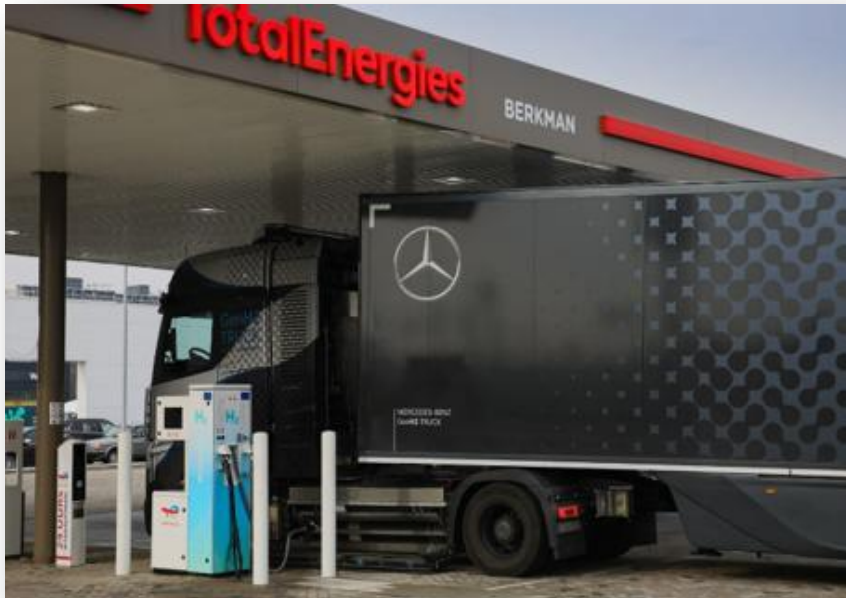
↑ Mercedes-Benz GenH2 prototype running on gaseous hydrogen, being refuelled at TotalEnergies station
